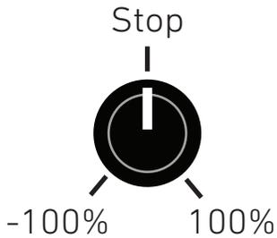
**SPEED:** -100% to +100%—Tape speed effect. Smoothly changes the playback speed, from forward (clockwise) to reverse (counter clockwise). In the middle, the sound is stopped. Reverse playback will play short segments of audio backwards, simulating studio tricks where a tape is flipped over to create a reverse guitar solo. The Tensor analyzes your playing to automatically adjust the size and timing of the reversed segments (See **NXT** hold mode or “Drift” if you need more control).
