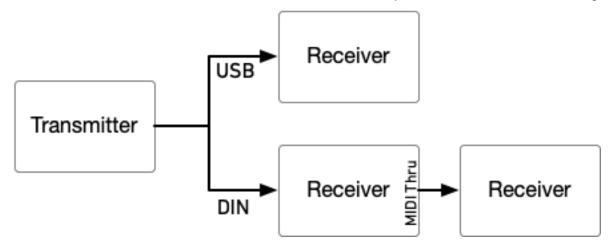
every quarter note (24 PPQ) and the receivers each calculate the tempo independently. Start, stop, and continue messages are used to synchronize playback between devices. The transmitter
