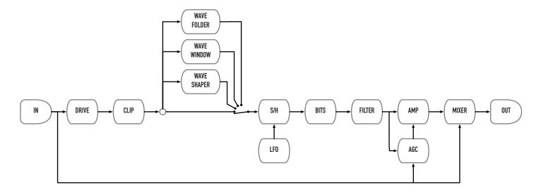
Bit crushing and waveshaping are amplitude-dependent effects, so it is helpful to be familiar with gain staging. Gain staging is adjusting the signal level at each point in the signal path - usually to maximize signal-to-noise ratio without distortion. In this case, we adjust the signal level to get different effects.
