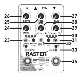
Hold down **WAVE/[ALT]** button to edit secondary parameters. Right LED will turn cyan. Settings are saved to presets and remembered when power is off. Knobs at center to turn off.
